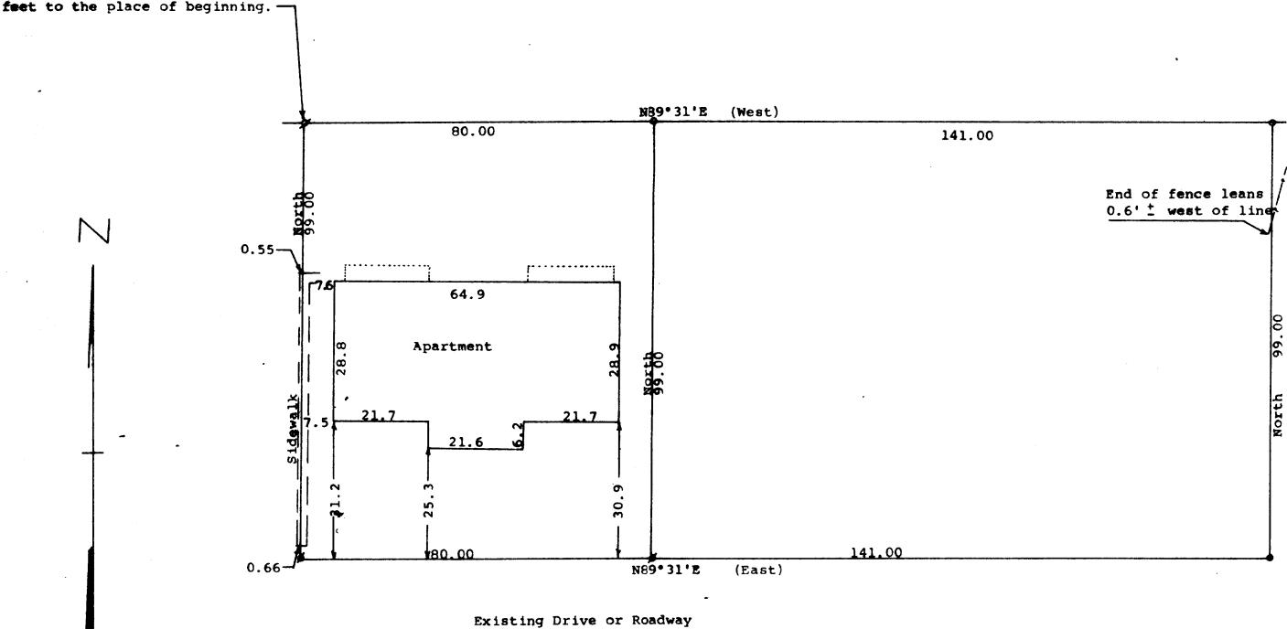
Scale - 1" = 20' # = 1 Iron Pipe Found 0 = 3/4" Iron Pipe Found • = 14" X 4' Iron Pipe Found bent and reset 14" X 24" iron pipe
